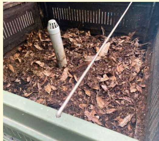
Figure 7 : Eartha model lane composter at Kasturba Nagar ( left ) ; Picture showing the interior of the Eira composting unit with the PVC aerator pipe ( right )
