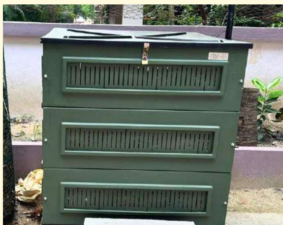
Figure 13 : Eira lane composters and dry leaves storage at Kasturba Nagar. A lock on the lid of the unit can also be seen here. The composting unit is kept locked in between layering and waste deposition to prevent misuse like dumping mixed waste
