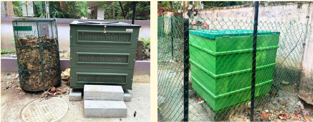
Figure 12 : Anterior view of the Eira (left) and posterior view of the Eartha (right) lane composters in Kasturba Nagar, Adyar. The Eartha composter ( left ) is seen here inside a mesh enclosure made of metal. The metal wire mesh enclosure acts as a protective measure to prevent misuse of the unit as well as a way to secure any extra tools. Other tools needed for the composting process are detailed at the end of this chapter (on page 56)
